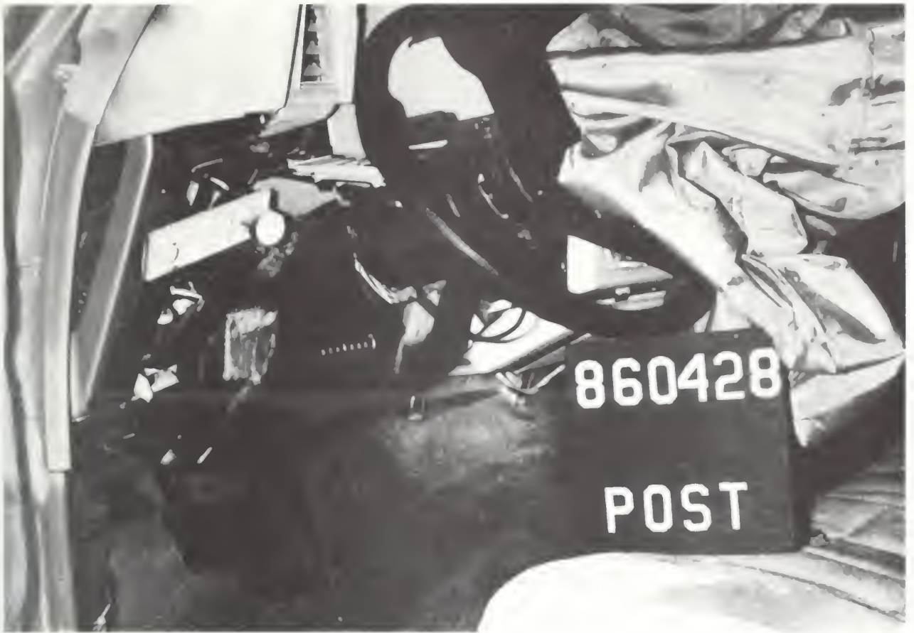
Figure A-21. POST-TEST STEERING COLUMN
